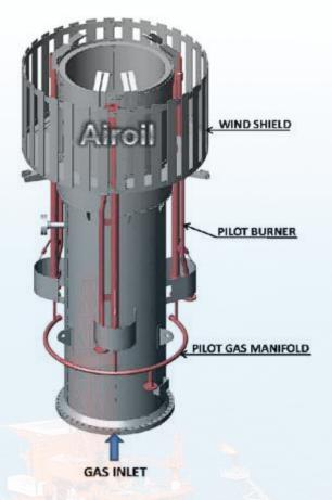
The Non-Smokeless flare tips are used where the environmental condition allows the burning of smoke producing gases. They are also used with gases which produce either no smoke or so little that smoke suppression with steam, air or high-pressure gas is not required. Examples of gas used with these tips are Hydrogen, Blast Furnace waste gas, Coke Oven gas, Ammonia, Hydrogen Sulphide and Methane.
