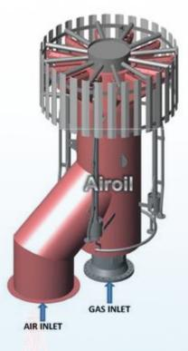
The Air-Assisted Smokeless Flare Tip is used for smokeless combustion applications, where the use of steam is not desired. Smokeless combustion can be obtained even with heavy unsaturated hydrocarbon gases.
