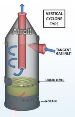
The Knock out drum is a vessel in the flare header designed to remove & accumulate condensed & entrained liquids from the relief gases.
