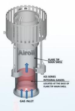
The Velocity Seal, located integrally at the base of the flare tip, has been designed to prevent air ingress into the flare system and has a number of advantages over gas inversion seals.
