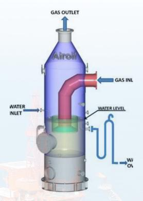
The purpose of a liquid (commonly water) seal drums in a flare gas system in threefold: -
